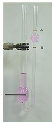
Capillary rise due to surface tension.
