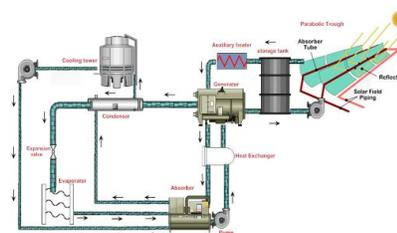
Experimental Set Up – Solar Powered Absorption Chiller Air Conditioning System
