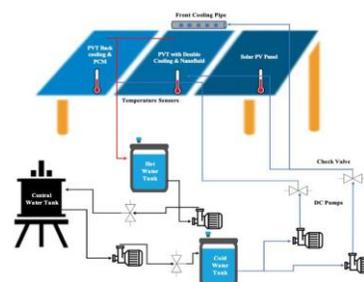
Experimental setup of hybrid PV-thermal collector with different cooling strategies
