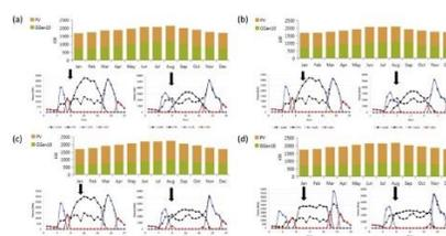
Monthly and daily average power outputs of HES for all proposed cases: (a) fixed, (b) CHA, (c) CVA, (d) dual-axis tracking.
