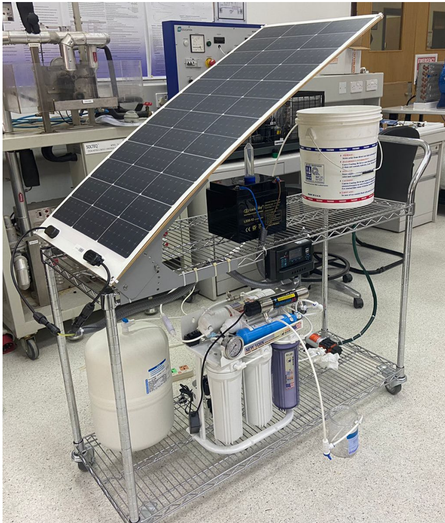
Figure 1: shows the solar-assisted water purification system prototype
