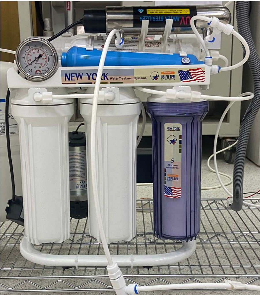
Figure 2: shows the filtration system utilized in the prototype
