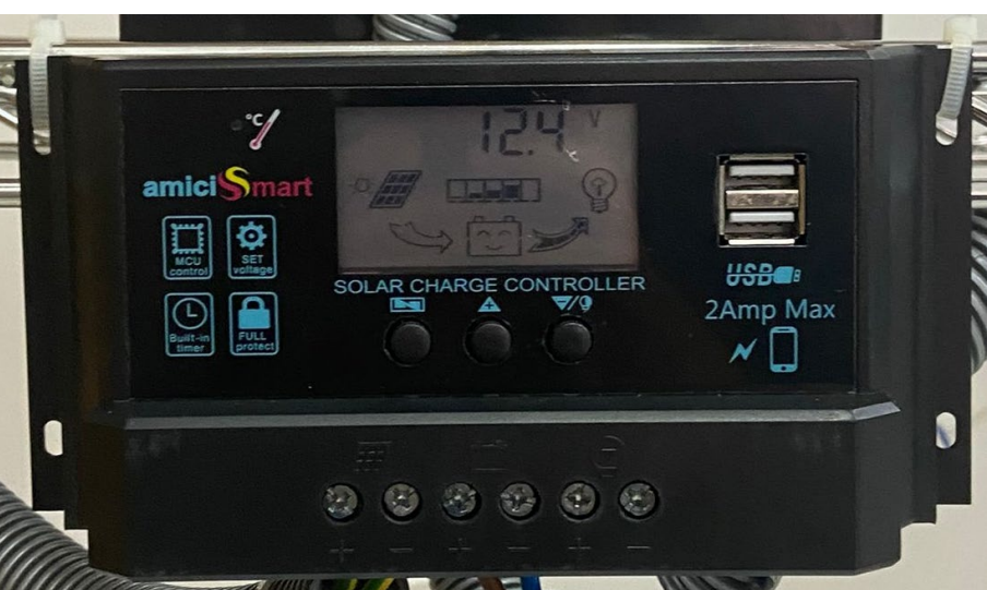
Figure 4: shows the solar charge controller when the system is activated
